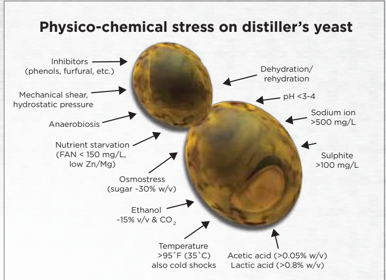
Figure 1: Ethanol plant operators must monitor these stress factors through all phases of fermentation or production can be compromised.
