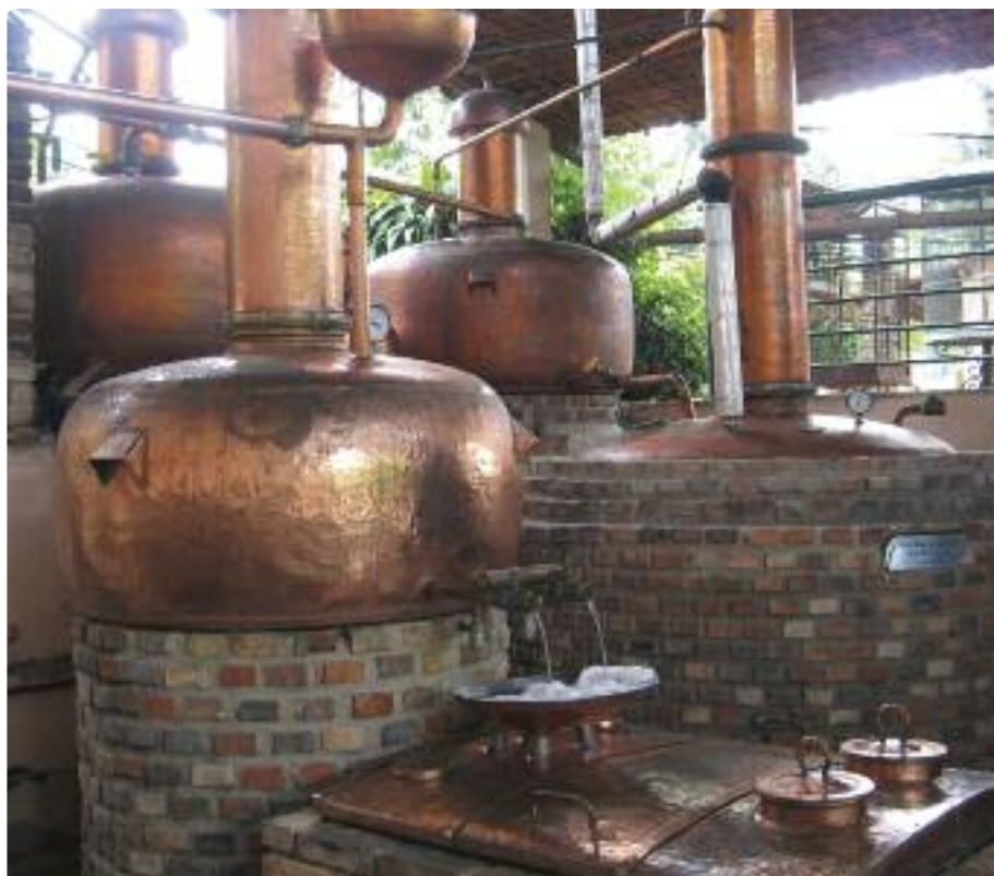
Alembic stills being used in the production of Cachaça in Brazil.
